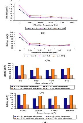
Fig. 5 Effect of (a) frequency, (b) amplitude, (c) gap voltage, and (d) capacitance on the percentage of short-circuit pulses
