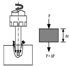
Fig. 3 Schematic diagram representing the pressures exerted in a micro fluid cell during the reduction of gap distance.
