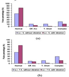
Fig. 6 Various pulse types in micro-EDM drilling of micro holes without and with the assistance of vibration at V=100 V and C=10 nF for(a) aspect ratio 5 and (b)aspect ratio 7.5
