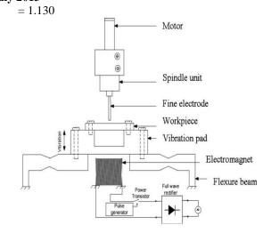
Fig. 4 Schematic diagram of the developed vibration unit
